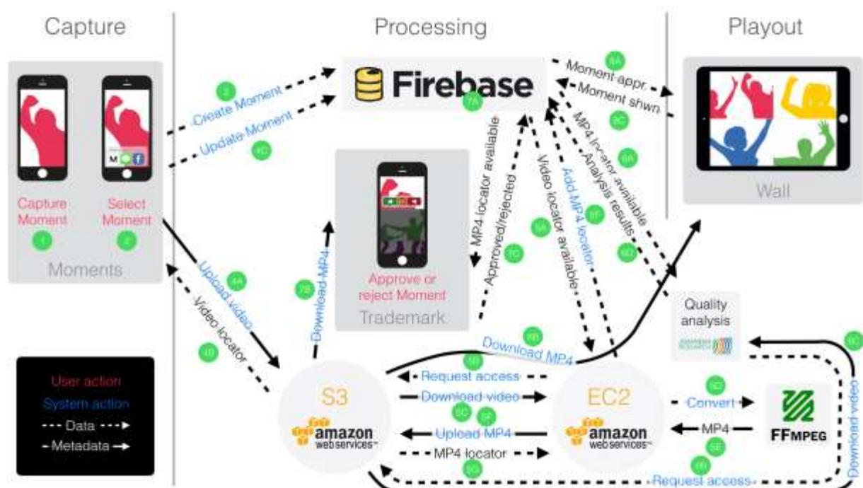
Figure 5: Wall of Moments system diagram
