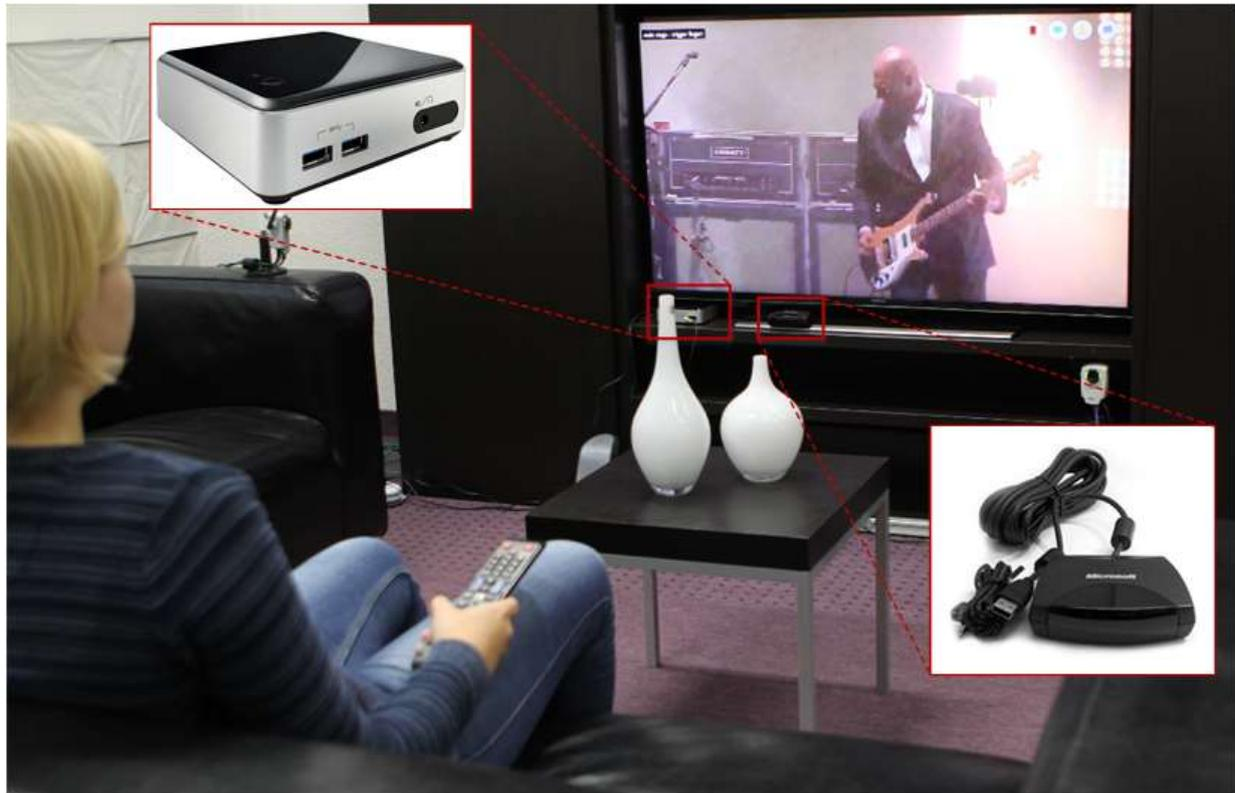
**Figure 7: WanderCouch deployment using an Intel NUC as set-top box emulator (on the left) and using an infrared receiver (on the right) to capture RC input.**
